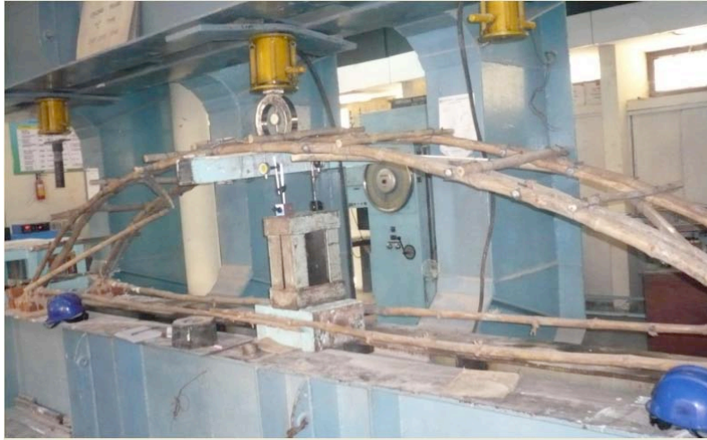
Figure 1 (a) Experimental Setup for bow beam without lateral support
