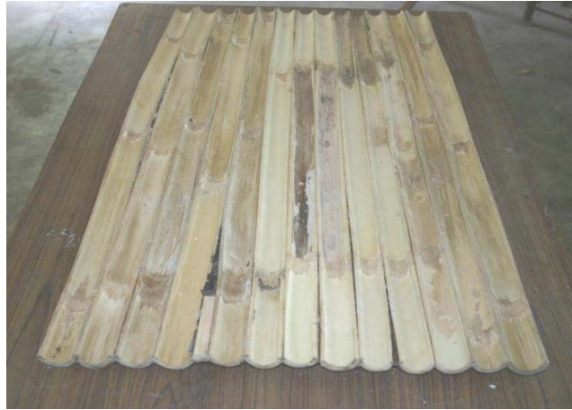
Figure 3 (b) Half split bamboo joined by fevicol and saw dust
