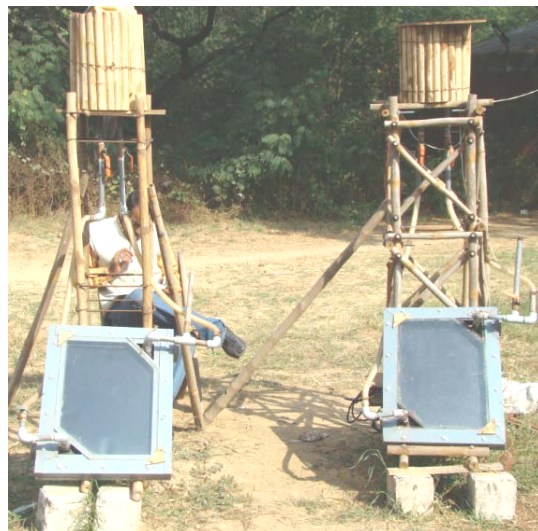
Figure 3 (f) Half split bamboo panel harvesting the solar energy
