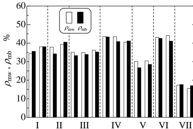
Figure 5. Measured solar reflectance of cool paints on parking lot
