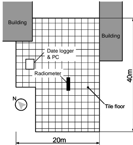
**Figure 2. Schematic drawing of location of tile surface for measuring reflectivity**
