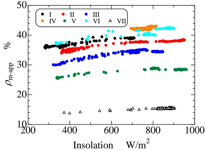
**Figure 6. Effect of global insolation on instantaneous apparent solar reflectance**
