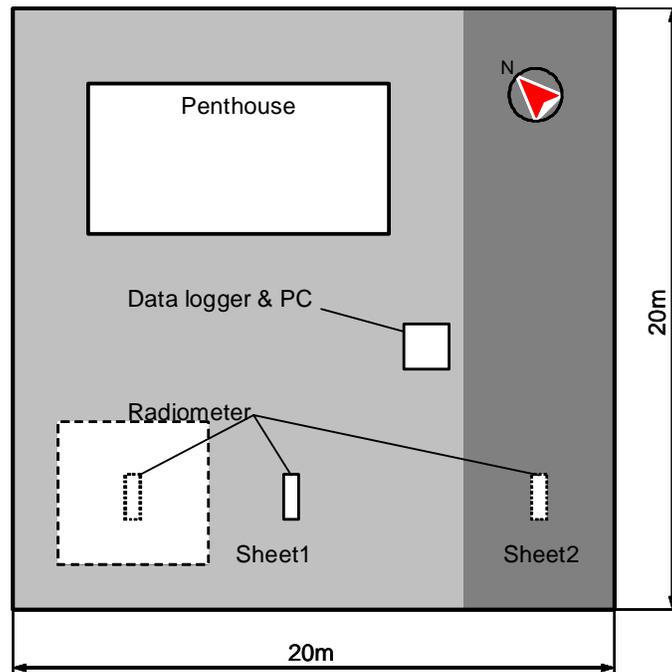
**Figure 9. Schematic drawing of waterproof sheet surface of a building rooftop and measuring areas**
