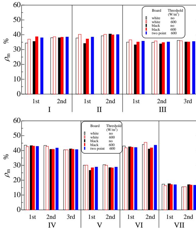
**Figure 7. Effect of data selection with threshold of insolation on solar reflectance**
