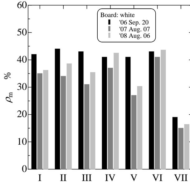
**Figure 8. Aged deterioration of each cool paint surface**
