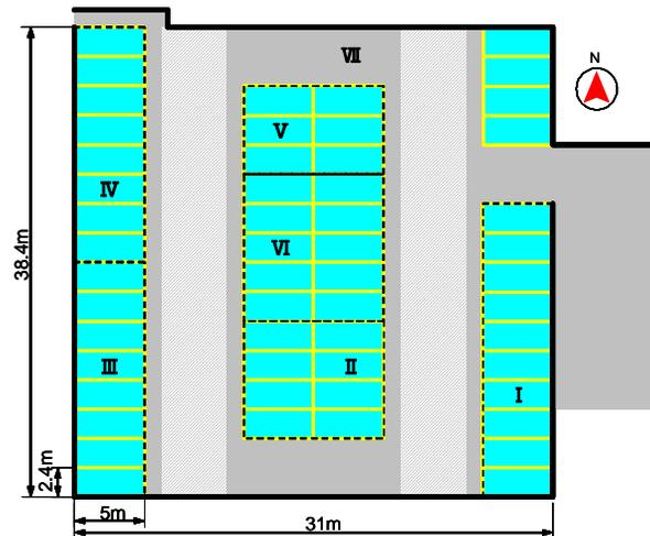
Figure 4. Schematic drawing of cool paint surface on rooftop stage of a parking lot and measuring areas
